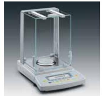
Sartorius LA analytical balance: precise weighing results, short measuring times, rugged in everyday laboratory use
