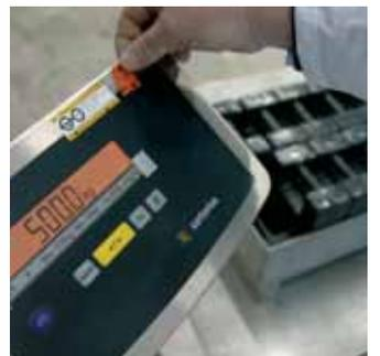
Issuing a German Calibration Service (DKD) calibration certificate with test mark
